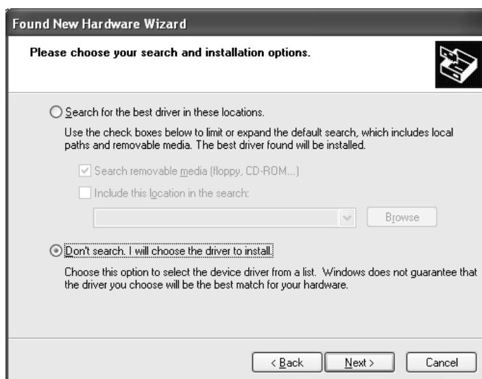
Pic. 7: Manual installation of drivers
